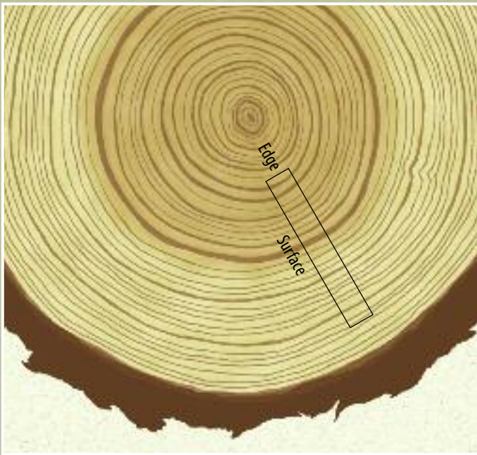
Boards are sawn at a radius across the growth rings. This creates long, vertical grain patterns on the surface of the lumber.
